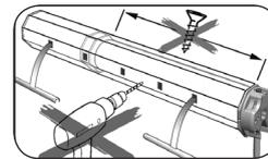
**Drilling and inserting screws in the area of the drive will cause the drive to be damaged.**
