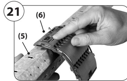
2. Slide the retainer profile for each shaft connector (6) onto the uppermost slat of the roller shutter (17).
