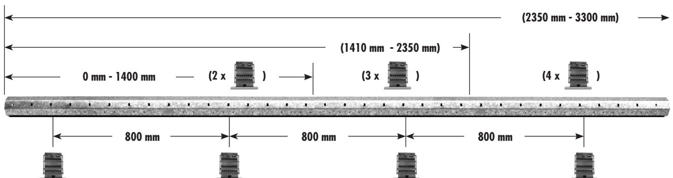
**Recommendation:** Mount an additional rigid shaft connector every 800 mm.
