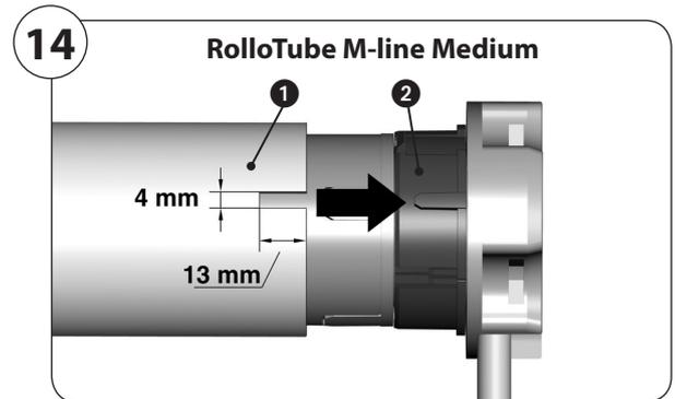
3. Slide the tubular motor into the precision tube.
