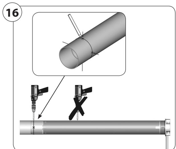
5. Screw or rivet the precision tube to the catch (8). Use four self-tapping sheet metal screws or four pop rivets for this.
