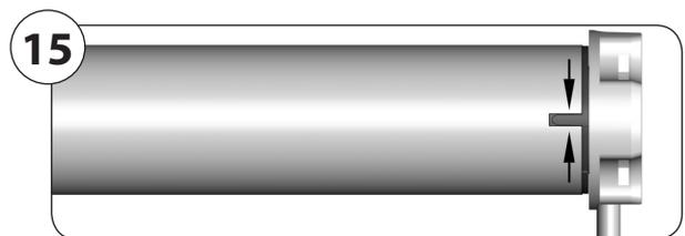
4. Mark the four fastening holes and subsequently drill them through the precision tube into the catch (8).
