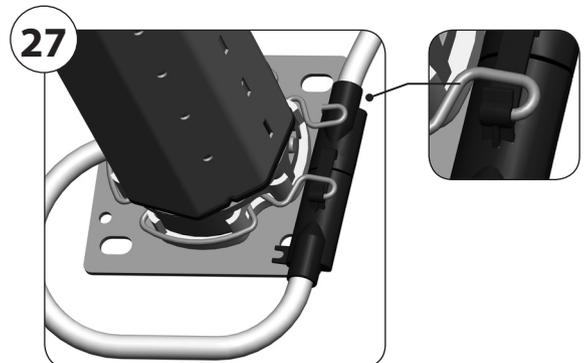
The retaining spring (14) should be rotated 90° to be plugged in and re-engaged.
