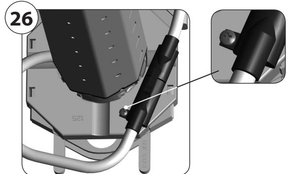
**Fixing the plug connection by clamping to the retaining spring of a click drive bearing:**
