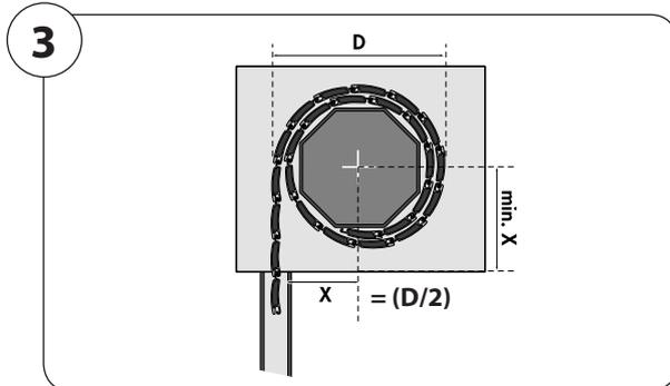
1. First determine the position of the drive (13) and counter bearing (1) in the roller shutter box.
