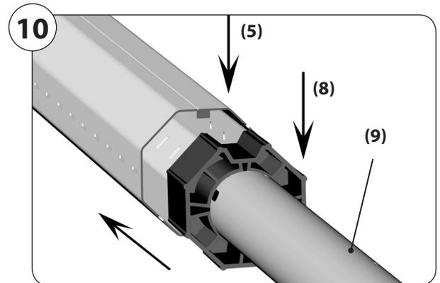
2. Subsequently, press the winding shaft (5) fully onto the adapter (10).
