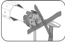
Inserting the tubular motor (9) forcibly into the winding shaft (5) will cause serious damage.
